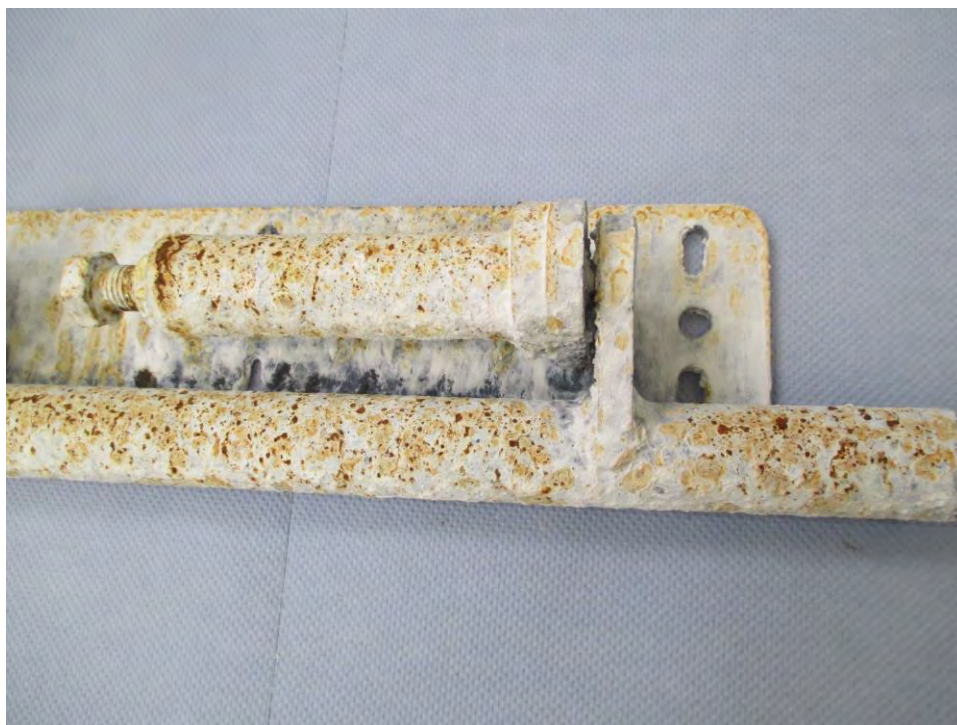
Fig 9: Photograph showing the condition of the Sample after 672 hours Salt Spray Test
