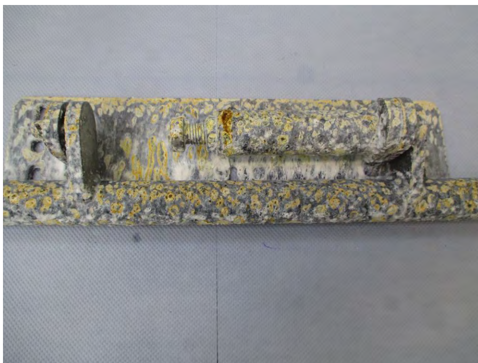
Fig 5: Photograph showing the condition of the Sample after 336 hours Salt Spray Test
