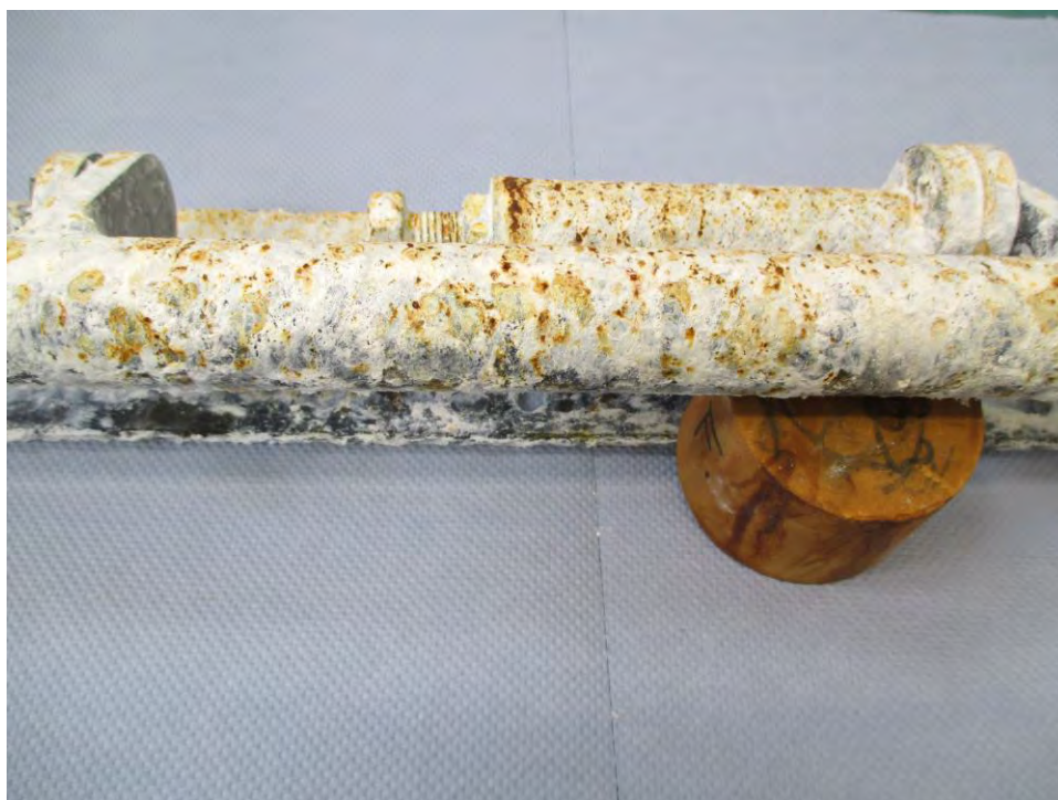
Fig 8: Photograph showing the condition of the Sample after 672 hours Salt Spray Test
