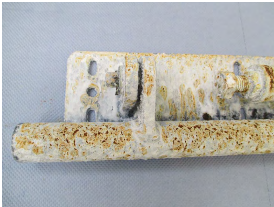
Fig 7: Photograph showing the condition of the Sample after 672 hours Salt Spray Test
