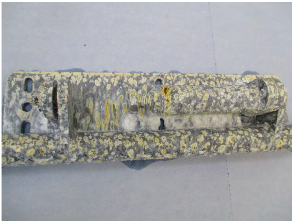
Fig 4: Photograph showing the condition of the Sample after 240 hours Salt Spray Test
