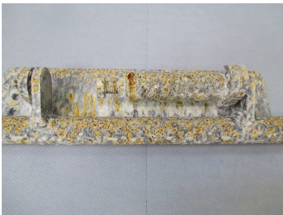
Fig 6: Photograph showing the condition of the Sample after 504 hours Salt Spray Test
