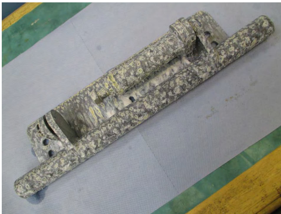
Fig 3: Photograph showing the condition of the Sample after 144 hours Salt Spray Test
