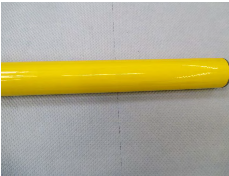
Fig 3: Photograph showing the condition of the 33.7 x 250mm Tube Sample after 216 hours Salt Spray Test
