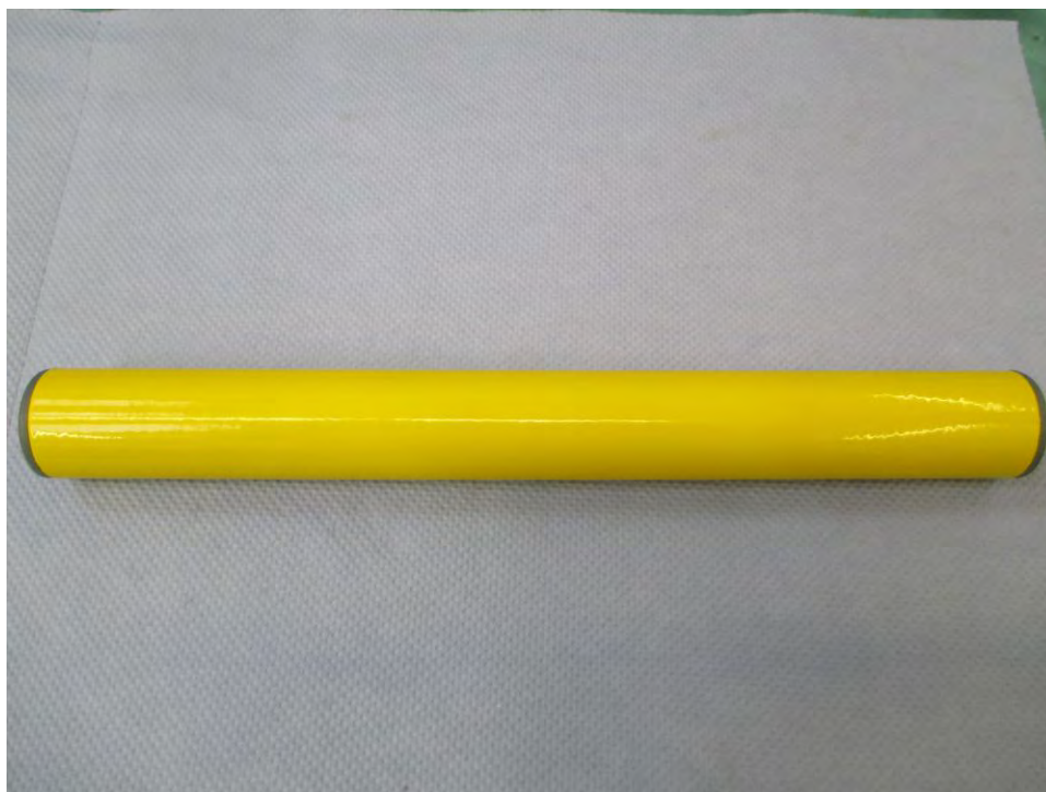
Fig 1: Photograph showing the condition of the 33.7 x 250mm Tube Sample prior to Salt Spray Test
