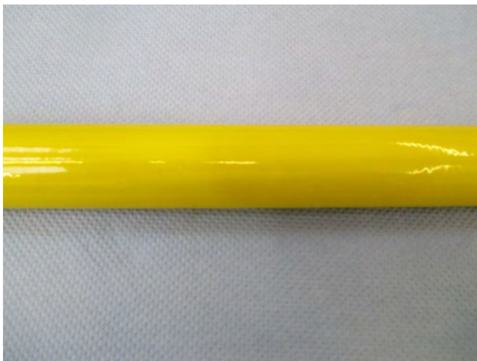
Fig 2: Photograph showing the condition of the 33.7 x 250mm Tube Sample
