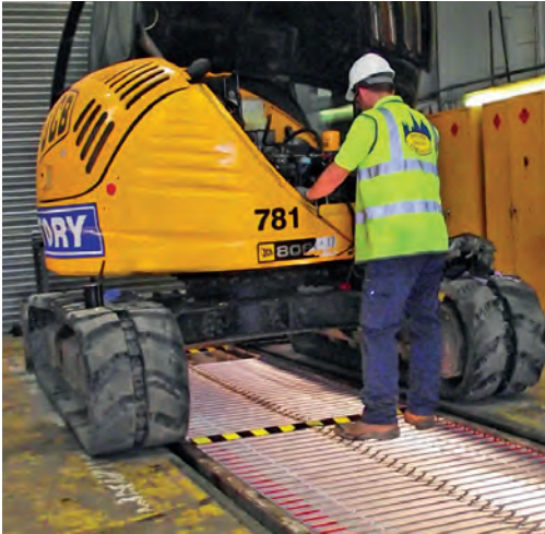
Prevents anyone from falling into the vehicle inspection pit in a transport workshop, whilst allowing full access to the vehicle underside.
