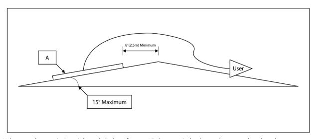
When used on an industrial steel clad roof up to 15 degree pitch, the anchor must be placed on the opposite pitch to the user at a minimum of 8 feet (2.5m) from the ridge.
