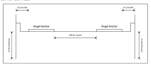
On a flat roof ensure that the Angel Anchor is a minimum of 8 feet (2.5m) from the edge of the roof.
